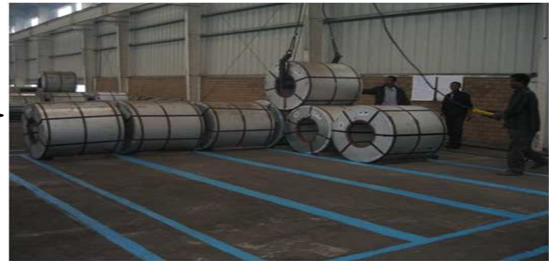
Fig. 2 In-process stock is repositioned to avoid Muda of transportation
